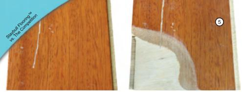
Engineered flooring has only a thin layer of hardwood that is glued to the top of a plywood base. This means that most engineered flooring is unable to be refinished. (5) Is an example of a piece of engineered flooring that was sanded down too far when it was being refinished. You can see the scratch penetrated all the way down to the plywood layer. When refinishing was attempted the top wear layer was totally removed by the flooring sander, which exposed the cheap plywood base.
